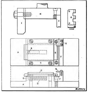
Fig. 13. Punch and Die for Curling a Hinge
